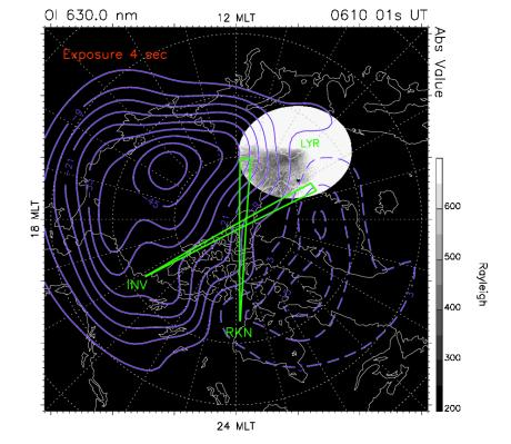
Figure 5 Image showing the 4-sec exposure time data at 0630 UT mapped onto the magnetic latitude and magnetic local time (MLT) coordinate system. Superimposed blues lines denote electrical potential contours derived from the SuperDARN data. The two green fan-shaped regions show the directions of beam 7 of the SuperDARN Inuvik and Rankin Inlet radars, respectively.
